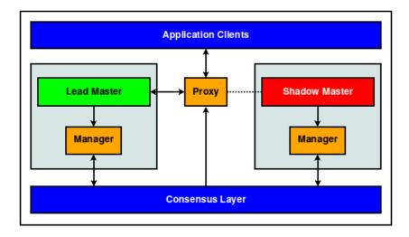
When using BDR as the HARP consensus layer, at least three fully qualified BDR nodes must be present to ensure a quorum majority. (Not shown in the diagram are connections between BDR nodes.)
