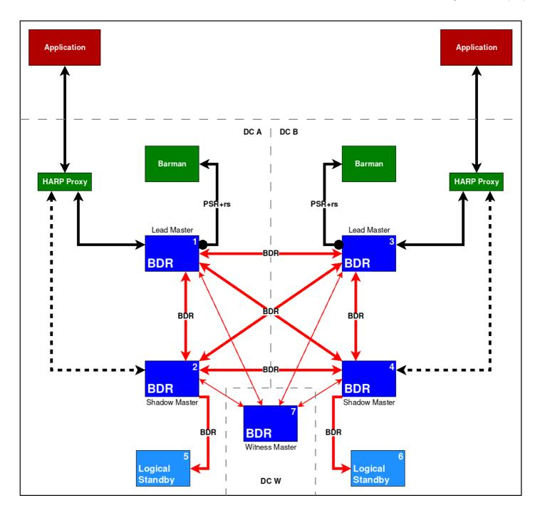
In this diagram, HARP Manager exists on BDR Nodes 1-4. The initial state of the cluster is that BDR Node 1 is the lead master of DC A, and BDR Node 3 is the lead master of DC B.
